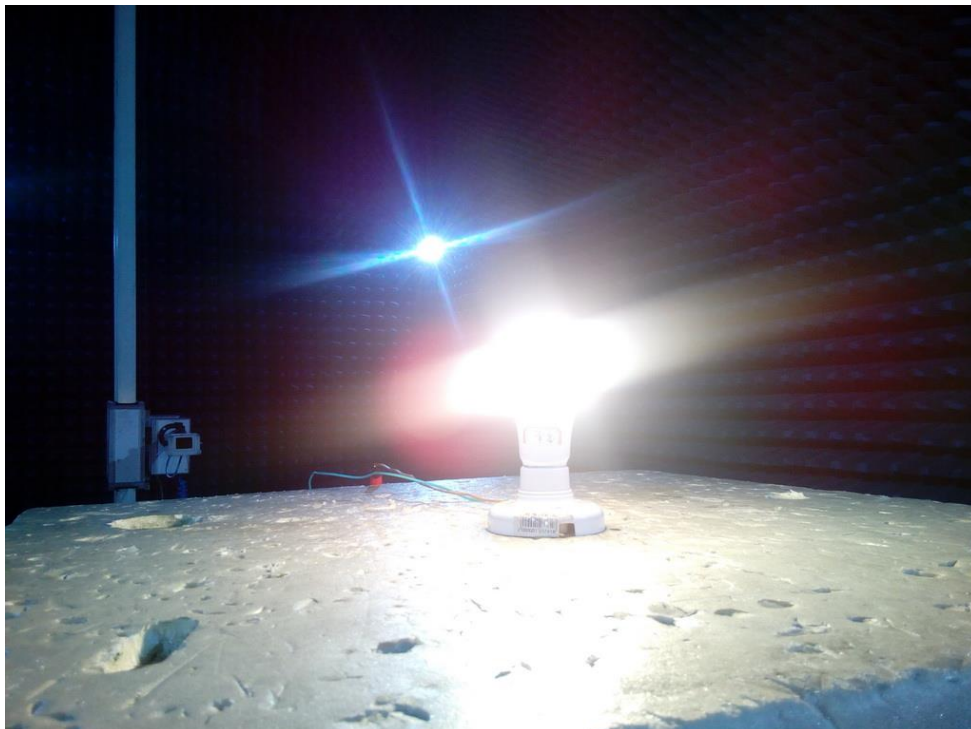
Photograph 4: Set-up for Radiated Spurious Emission (18GHz ~ 26.5GHz)
