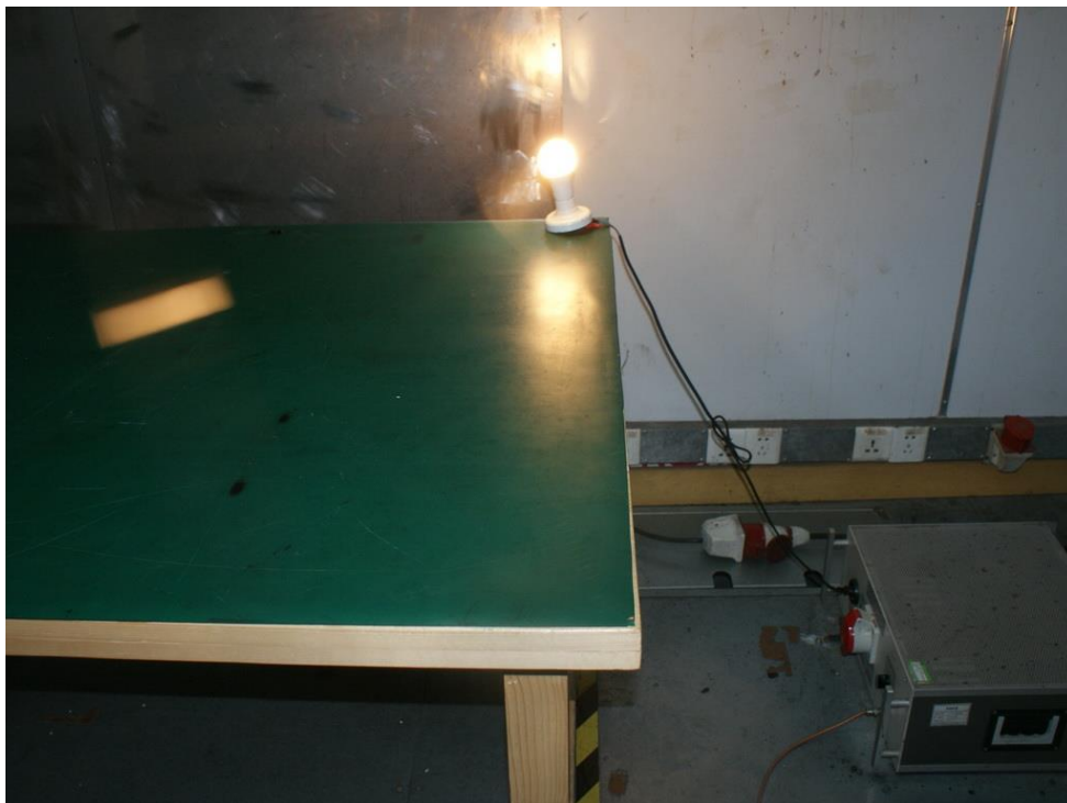
Photograph 6: Set-up for Conducted Emission
