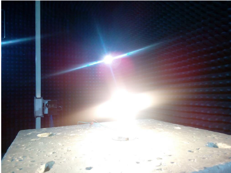
Photograph 4: Set-up for Radiated Spurious Emission (18GHz ~ 26.5GHz)
