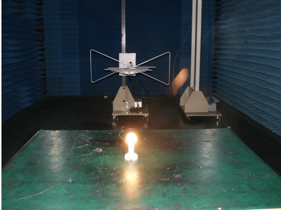
Photograph 8: Set-up for Radiated Emission (1GHz ~ 6GHz)
