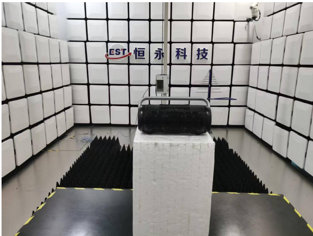
Radiated Test (Above 1GHz)
