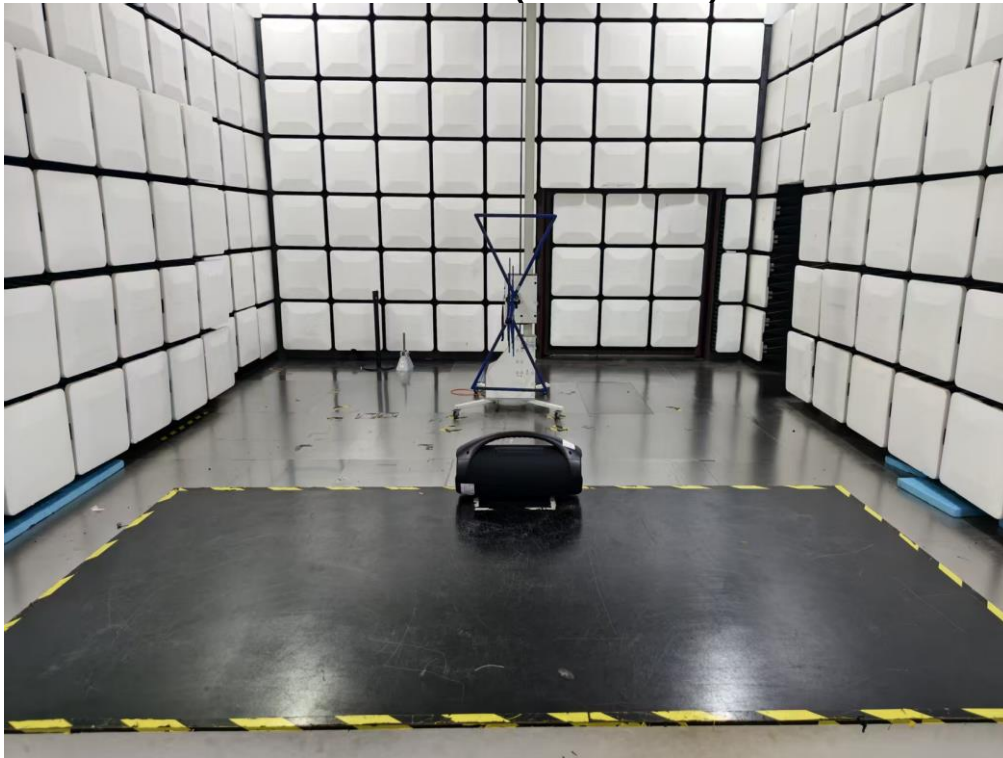
Radiated Test (Below 1GHz)
