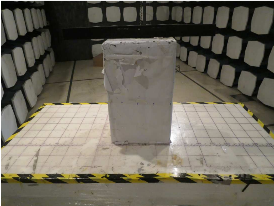
Front View of Radiated Emissions above 1GHz
