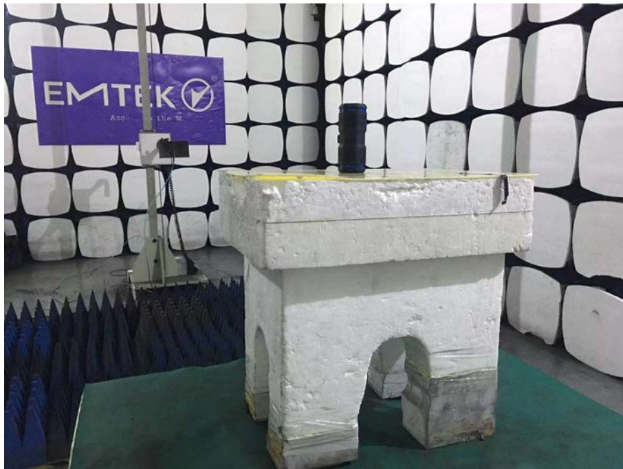
Spurious Emission Test Setup (Above 1GHz):
