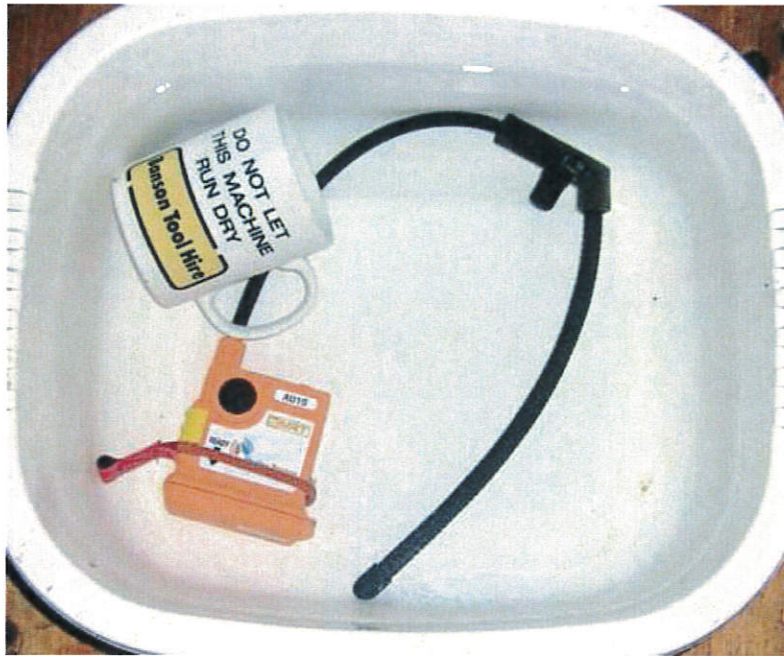
Figure A.1 – Thermal shock submersion in water
