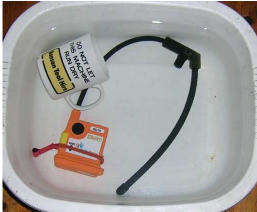
Figure A.1 – Thermal shock submersion in water
