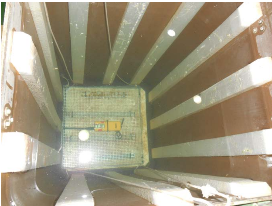
SPECIMEN TRA-021534-S2 SECURED TO A WEIGHTED FRAME FOR IPX7 IMMERSION
