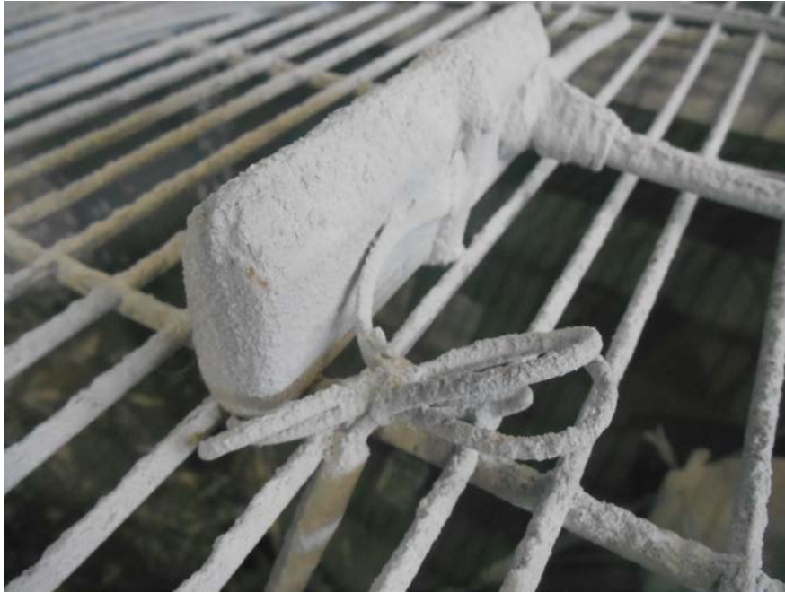
SPECIMEN TRA-021534-S1 AFTER UNDERGOING IP6X DUST TEST
