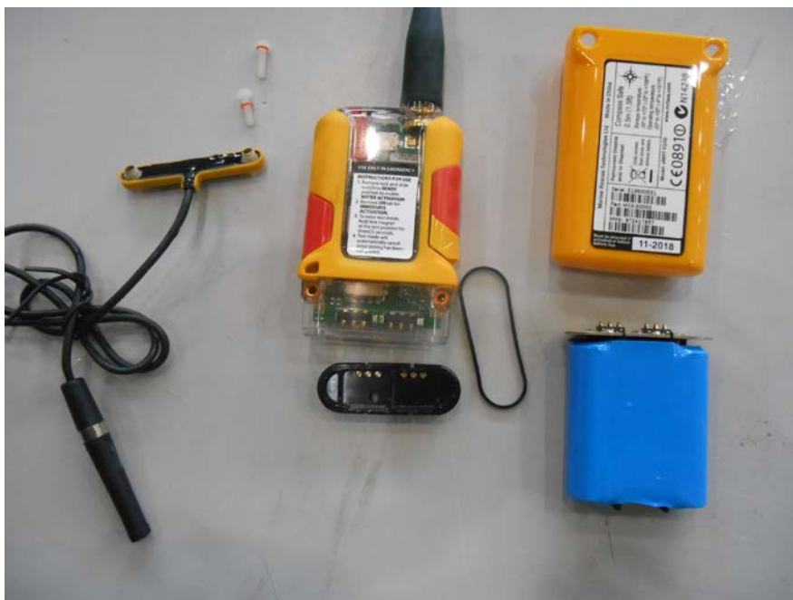
SPECIMEN TRA-021534-S2 INSPECTED FOR WATER INGRESS
