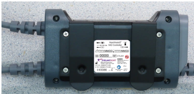
Figure 30- Belt clip fastened to the rear housing with label applied.
