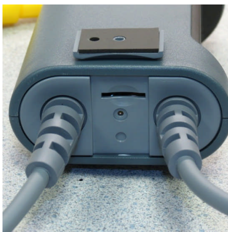
Figure 32- Right housing shown without the SIM card cover
