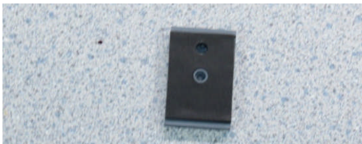
Figure 31- SIM card cover with gasket applied
