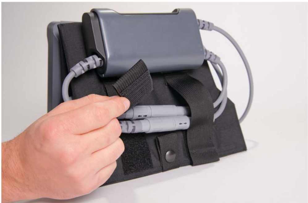
Figure 4-23. Securing the battery connectors in the VADPAK Insert
