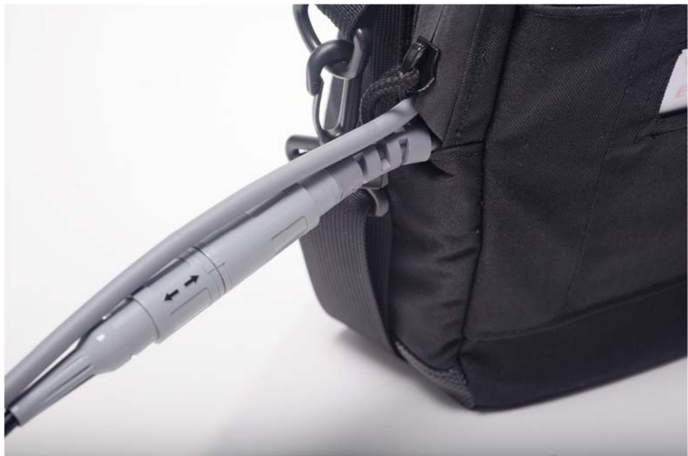
Figure 4-30. Routing the cables in the VADPAK
