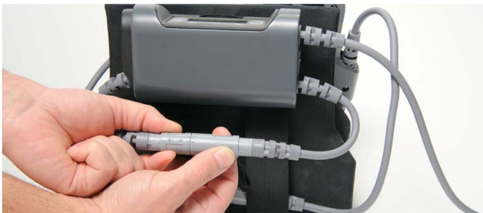
Figure 4-34. Batteries connected to the Controller
