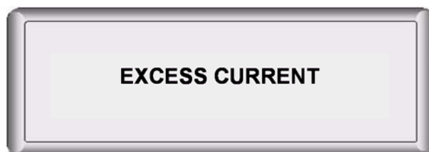
Figure B-11. Diagnostic alarm 1: EXCESS CURRENT
