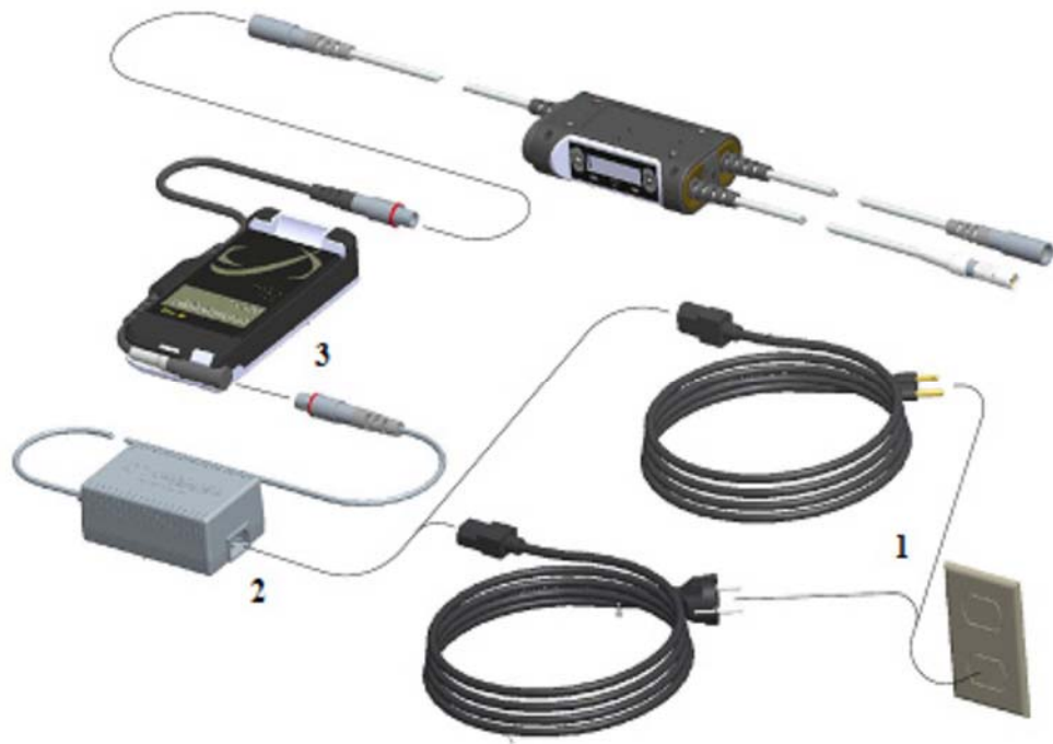
Figure 4-38. Independent Power Supply connection diagram
