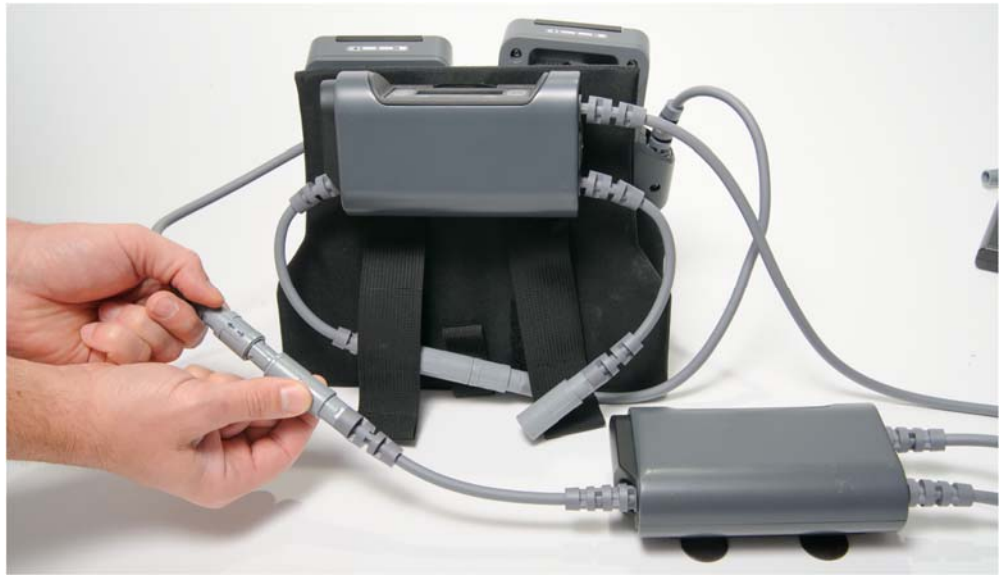
Figure 4-8. Connecting the first battery pocket to the backup Controller
