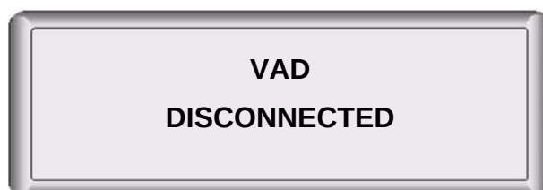
Figure B-10. Emergency alarm 3: VAD DISCONNECTED
