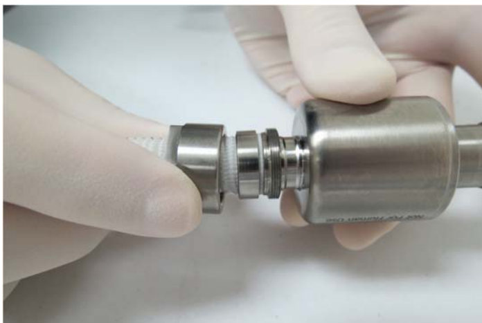
Figure 3-9. Sliding the wedge nut over the wedge
