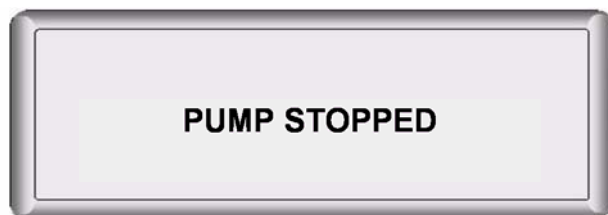
Figure B-8. Emergency alarm 1: PUMP STOPPED
