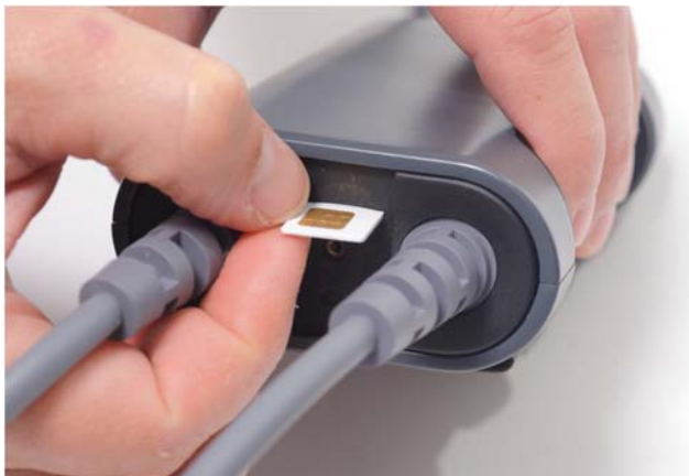
Figure 4-15. Removing the SIM card from the Controller
