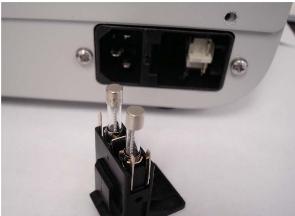
Figure 5-24. Fuse block in power inlet module
