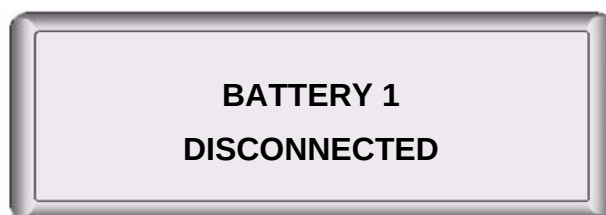
Figure B-15. Diagnostic alarm 5: BATTERY 1 DISCONNECTED
