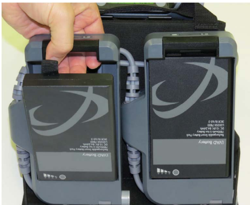
Figure 4-35. Removing the battery from the battery pocket
