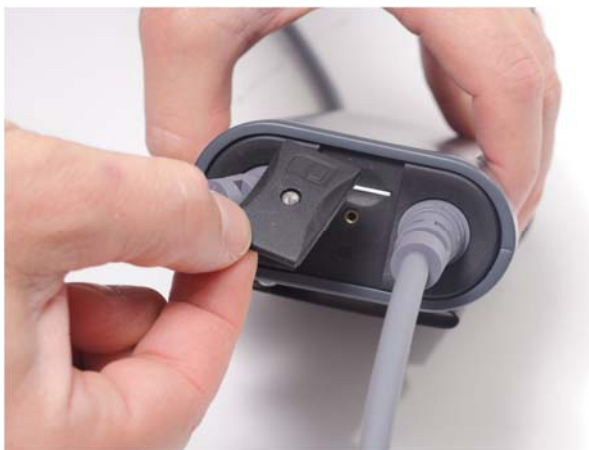
Figure 4-17. Replacing the SIM card cover
