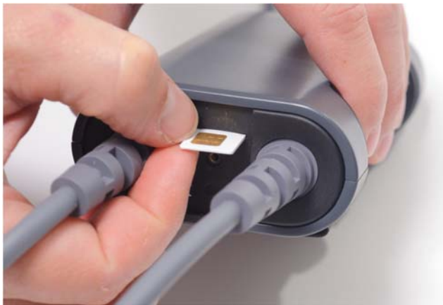
Figure 4-15. Removing the SIM card from the Controller
