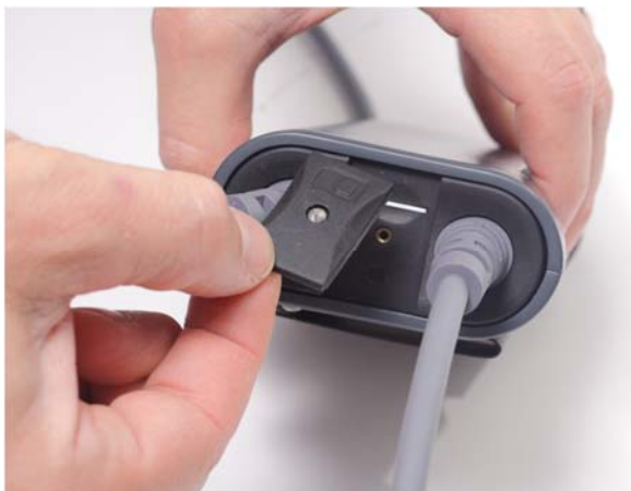
Figure 4-17. Replacing the SIM card cover
