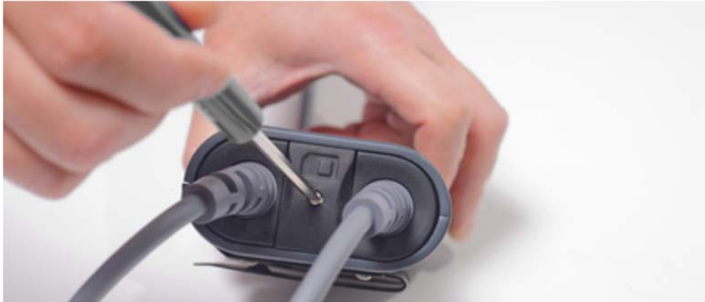
Figure 4-14. SIM card covers removed from both Controllers
