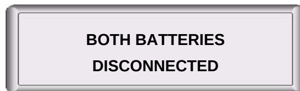
Figure B-9. Emergency alarm 2: BOTH BATTERIES DISCONNECTED
