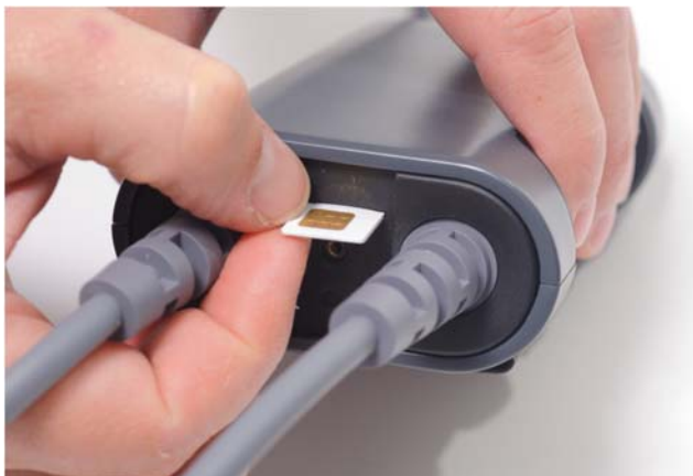
Figure 4-16. Inserting the SIM card into the backup Controller
