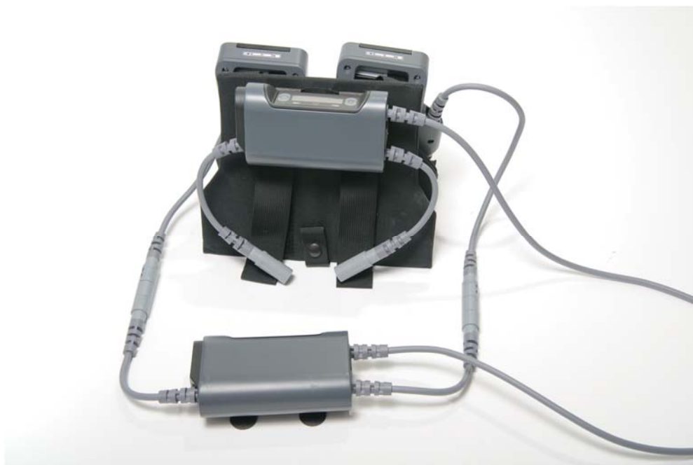
Figure 4-12. Connecting the second battery pocket to the backup Controller
