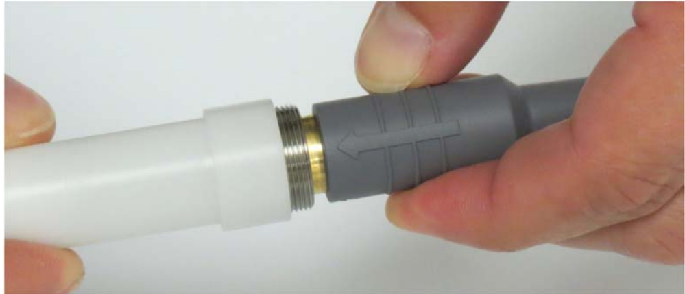
Figure 4-6. Unscrewing the defibrillation cover
