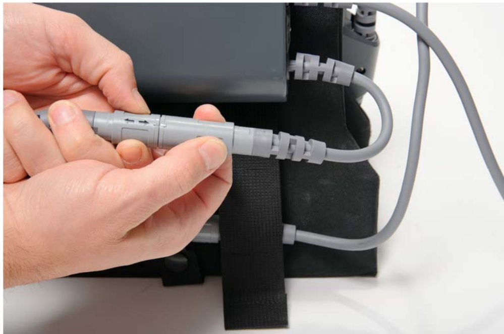
Figure 4-7. Disconnecting one battery pocket from the Controller
