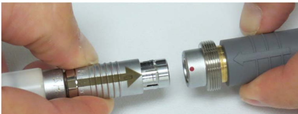
Figure 4-10. Aligning the driveline cable to the backup Controller
