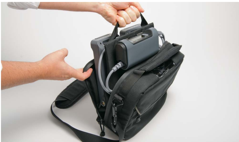
Figure 4-4. Removing the VADPAK Insert from the VADPAK
