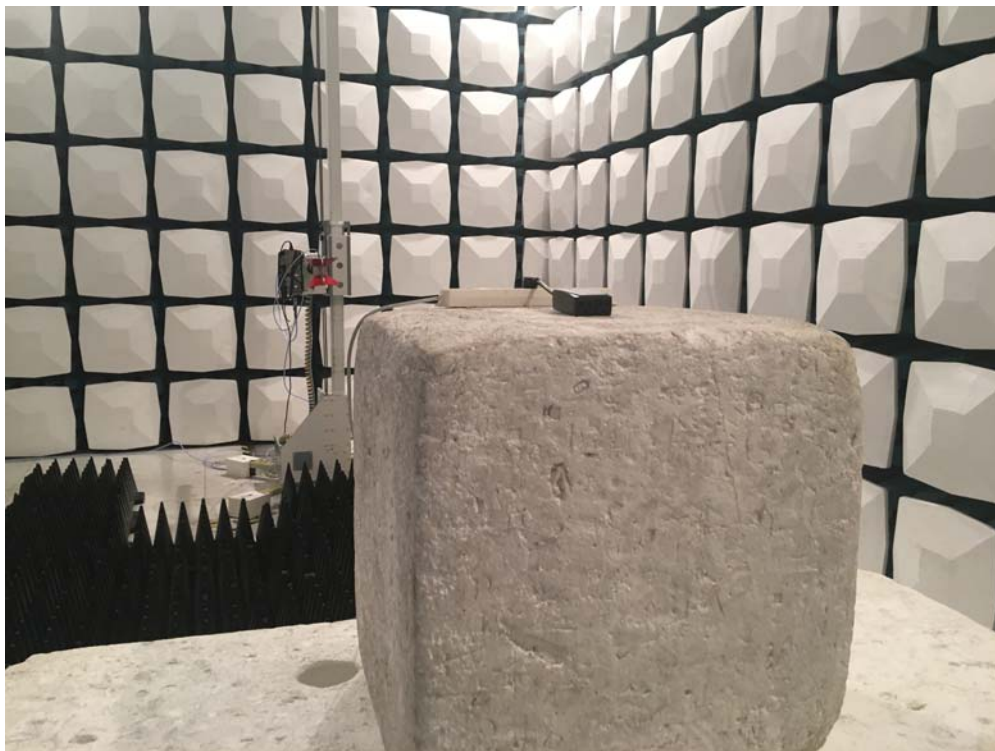
Description: Radiated Emission Test Setup for 1~18GHz
