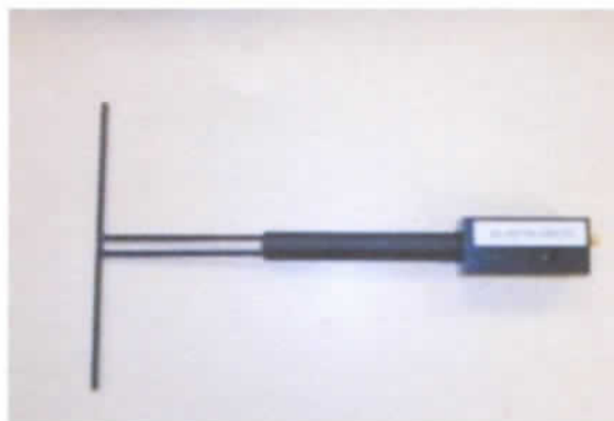
Figure 1 – Satimo COMOSAR Validation Dipole
