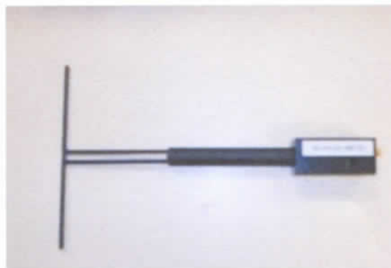
Figure 1 – Satimo COMOSAR Validation Dipole
