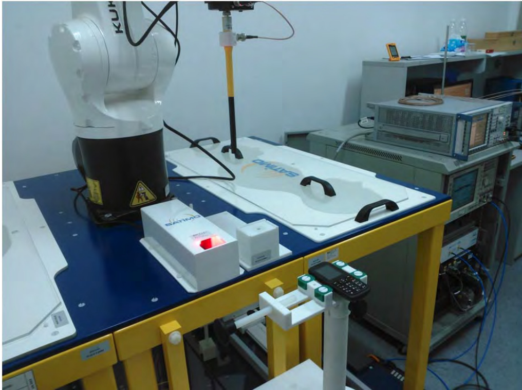
T-Coil Measurement Test Setup
