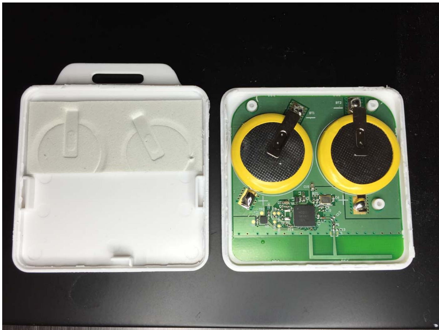
Figure 1 SwipeSense Badge, internal photo showing antenna at bottom of PWB
