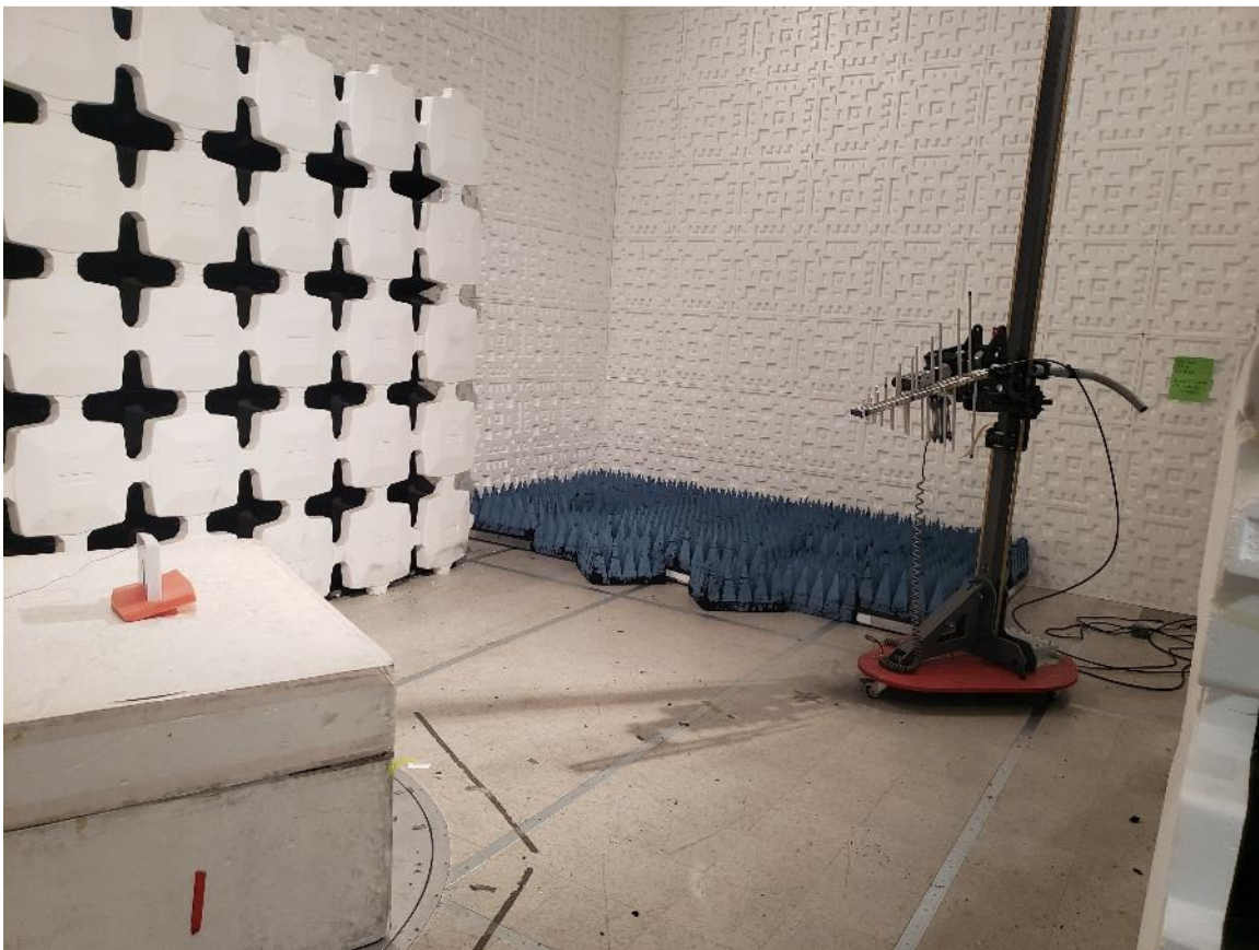
Figure 4. Radiated Emissions Test Setup, 200 MHz to 1GHz
