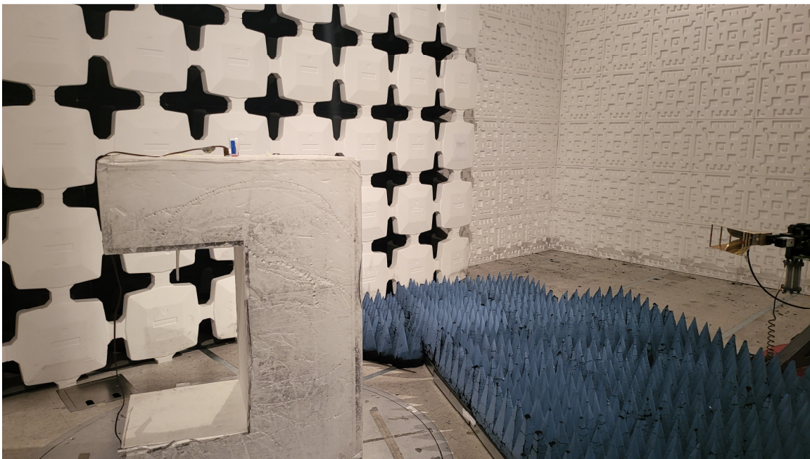
Figure 5. Radiated Emission Test Setup, above 1 GHz
