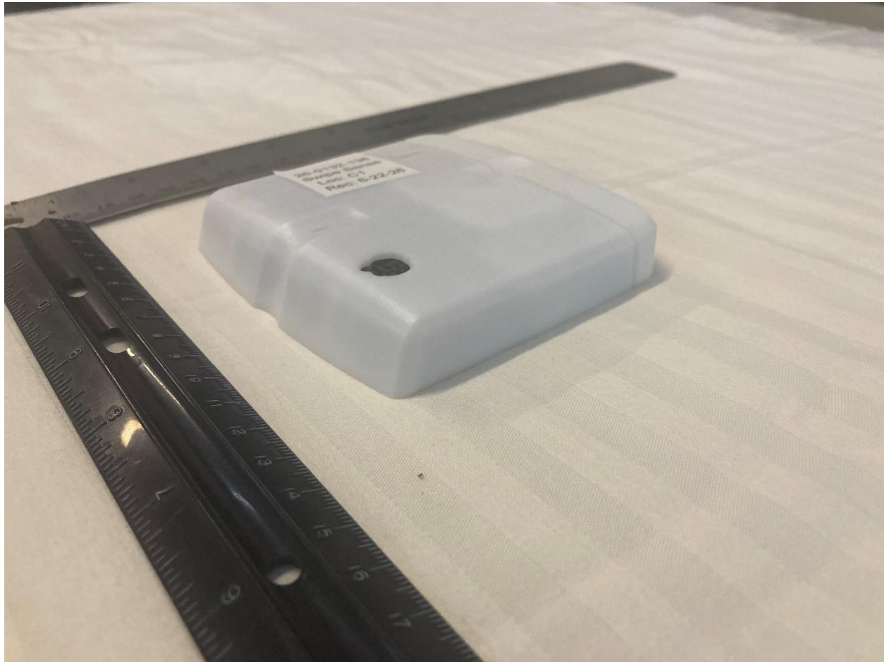
Figure 9. Side View with removable cover in place
