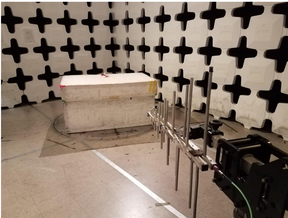
Figure 4. Radiated Emissions Test Setup, 200 MHz to 1GHz
