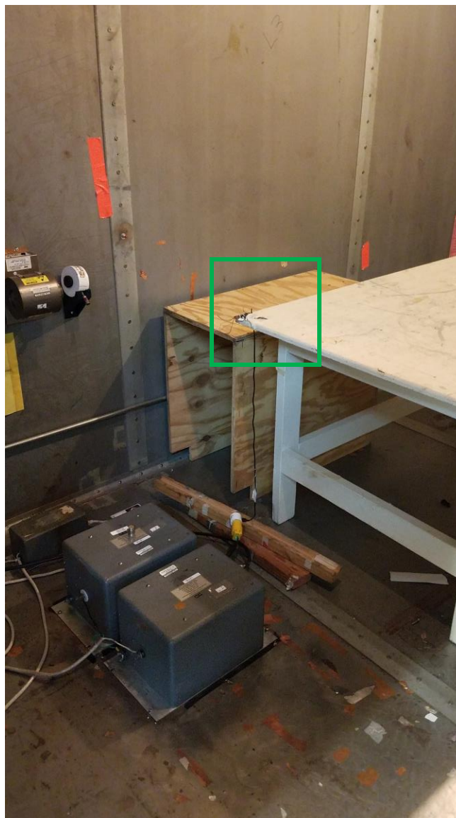
Figure 7. Powerline Conducted Emissions Setup
