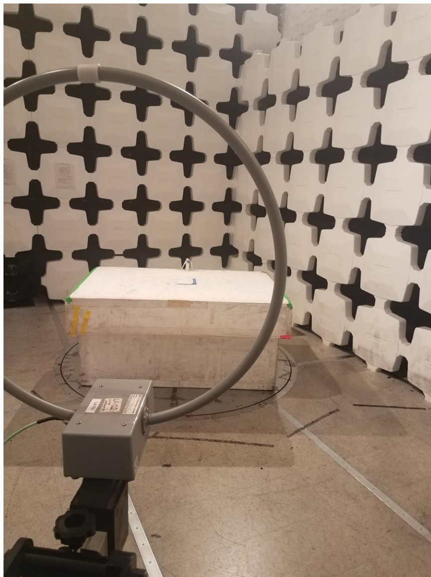
Figure 2. Radiated Emissions Test Setup, .15 MHz to 30 MHz
