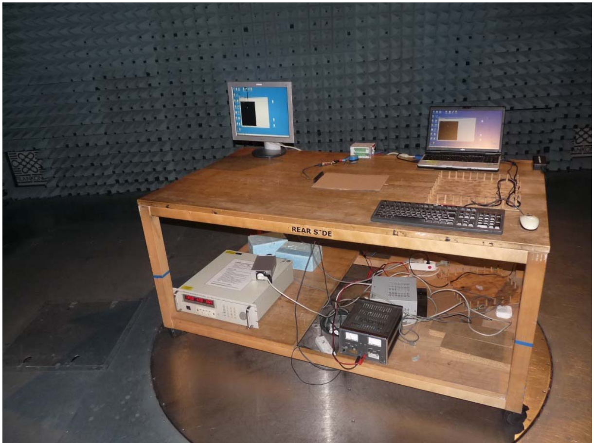
Photo 4: Test setup for radiated measurements, EUT in horizontal position EUT supplied by stabilized AD/DC power supply Computer peripheral setup Semi-anechoic chamber, 30 MHz to 1 GHz unintentional radiator §15
