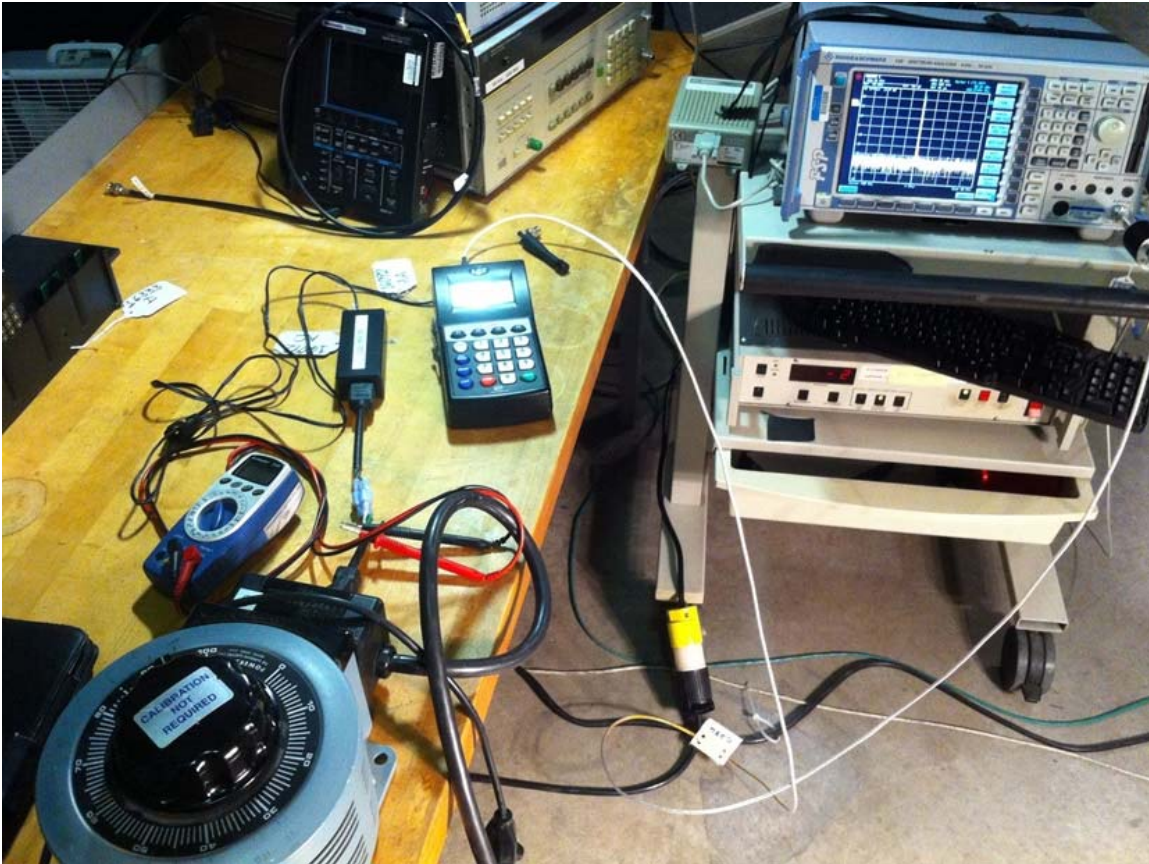
FREQUENCY STABILITY, VOLTAGE
