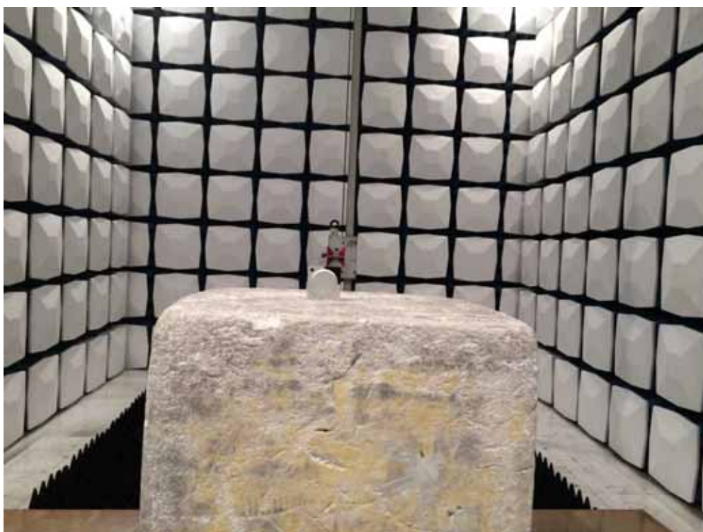
Description: Radiated Emission Test Setup for 1~18GHz
