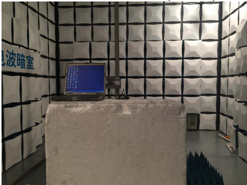
RADIATED RF MEASUREMENT SETUP (Above 1 GHz)
