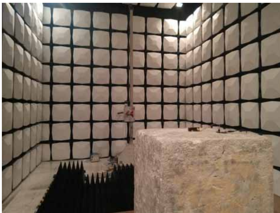
Description: Radiated Emission Test Setup for 18~25GHz
