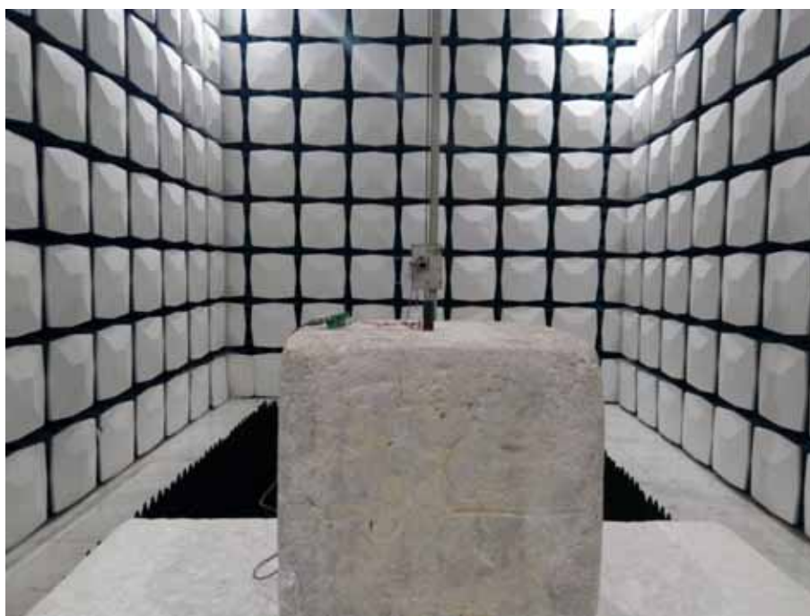
Description: Radiated Emission Test Setup for 18~25GHz
