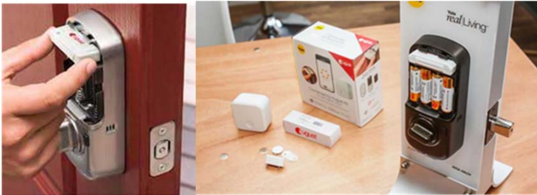
The MD-02 is installed above the battery compartment of the Yale lock.
