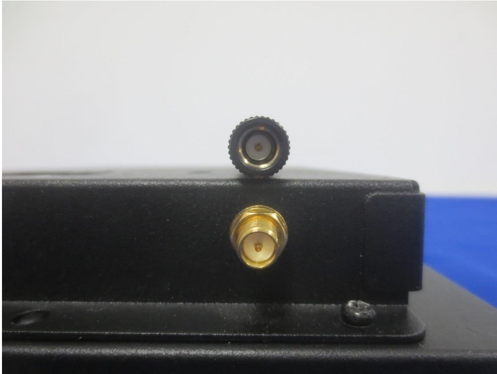
Note: Reversed polarity Non standard external antenna port
