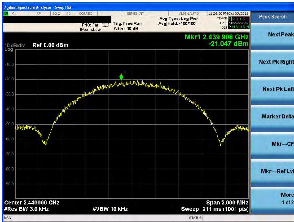
Power spectral density plot on channel 19
