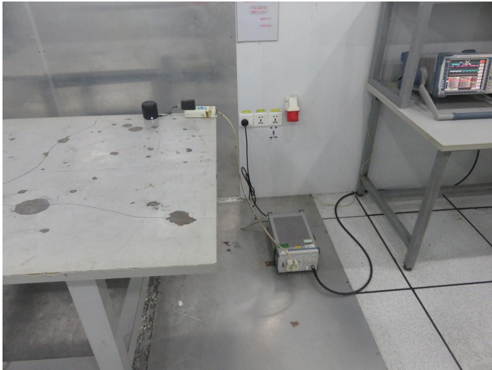
Photo of Conducted Emission Measurement
