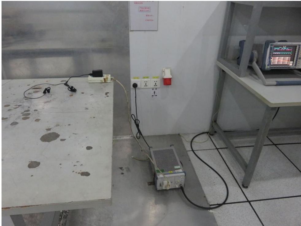
Photo of Conducted Emission Measurement
