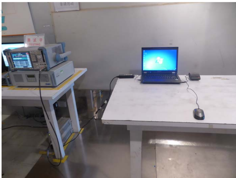
TEST SETUP OF CONDUCTED EMISSION
