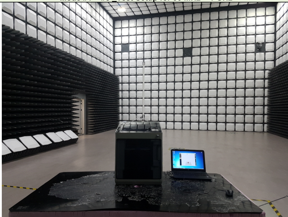
Mode #1 ~ #5 Test Setup for 30 MHz ~ 1 GHz
