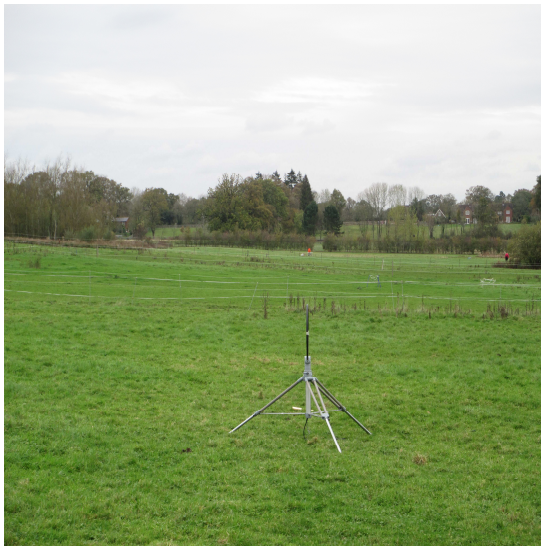
Set up for 300 metre measurements (mag loop end, orange in distance is EUT location)
