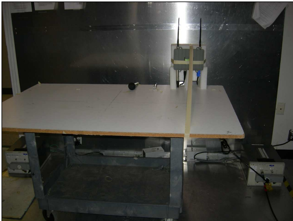
Figure 3: Test Setup Photo – Conducted Emissions – AiRocks Configuration
