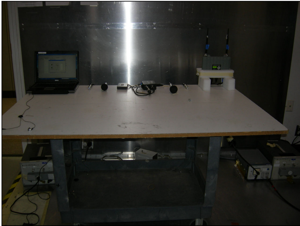
Figure 5: Conducted Emissions – AiRocks Configuration
