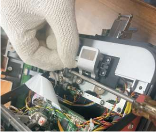
4. Put on cotton gloves and pinch the blade tightly with your hand (to avoid hurting your hand), then use a screwdriver to remove the blade
