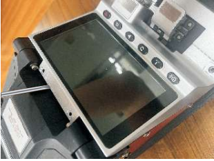
2. Use a flat screwdriver to gently lift the screen cover as shown in the figure, and then remove the screen cover
