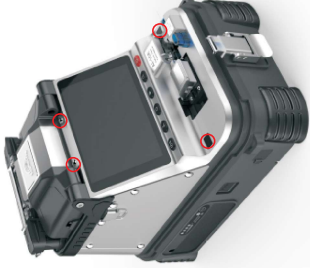
6. Replace the screen cover and secure the four screws shown in the figure. Blades change completed
