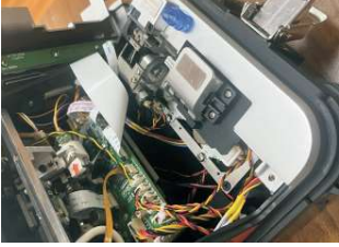
3. Place the screen cover on the side of the body, no need to remove the connecting wire
