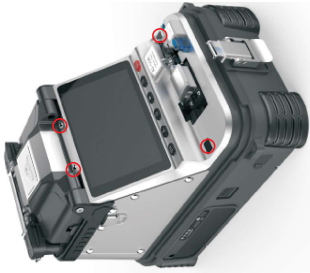
1. Use a Phillips screwdriver to remove the four screws at the red
