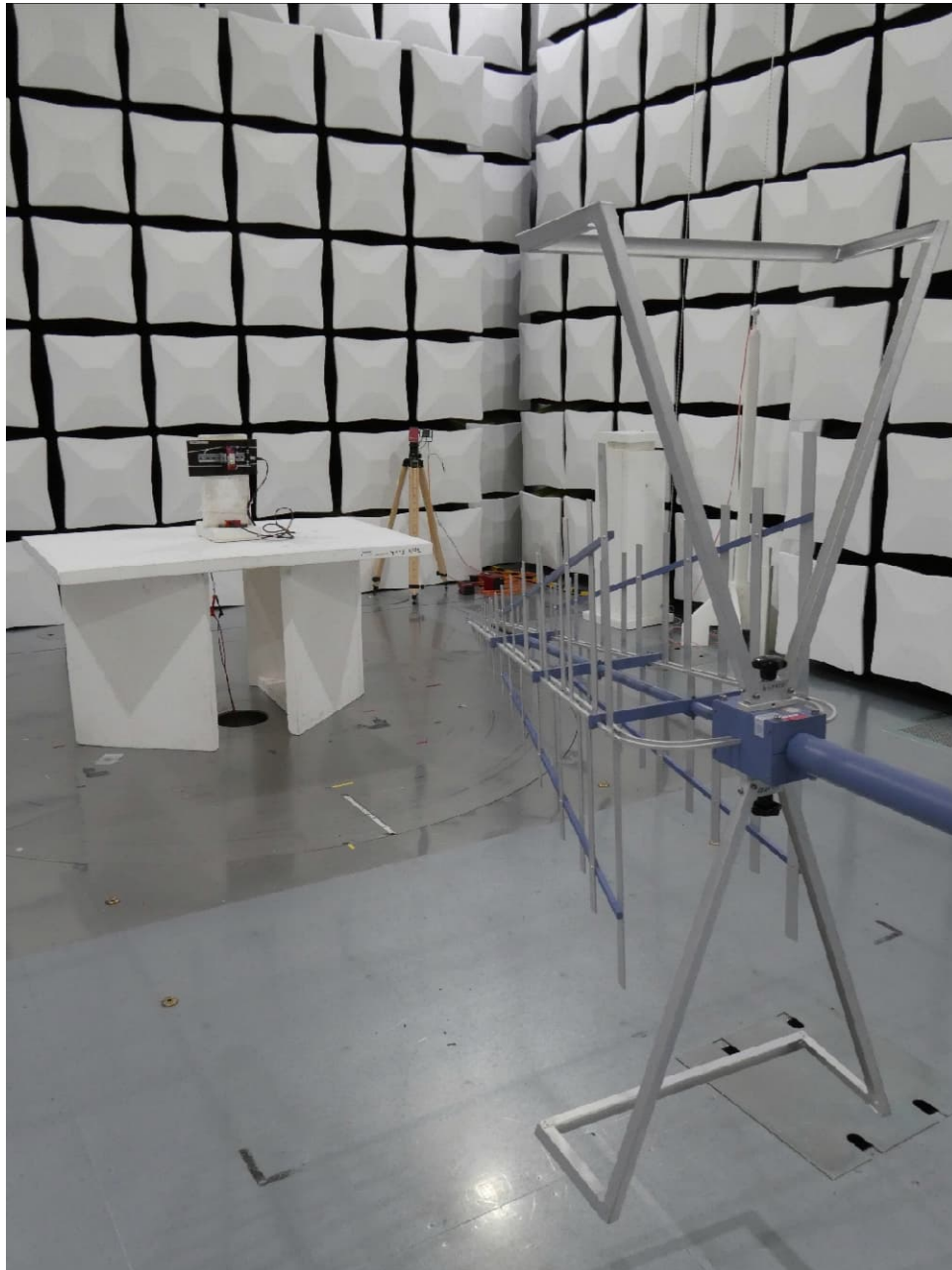
Test setup semi anechoic chamber <1 GHz
