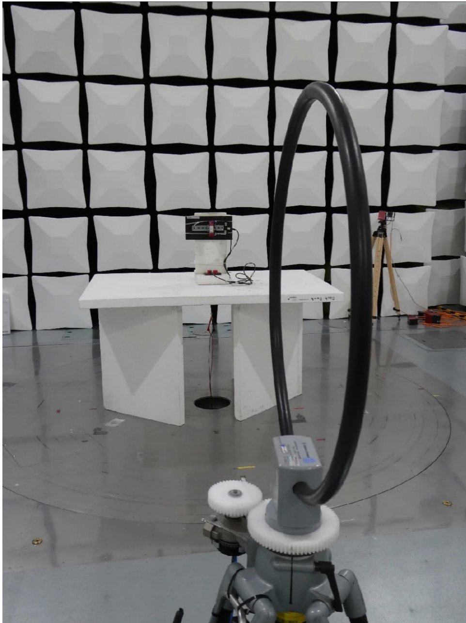
Test setup semi anechoic chamber <30 MHz EUT 2
