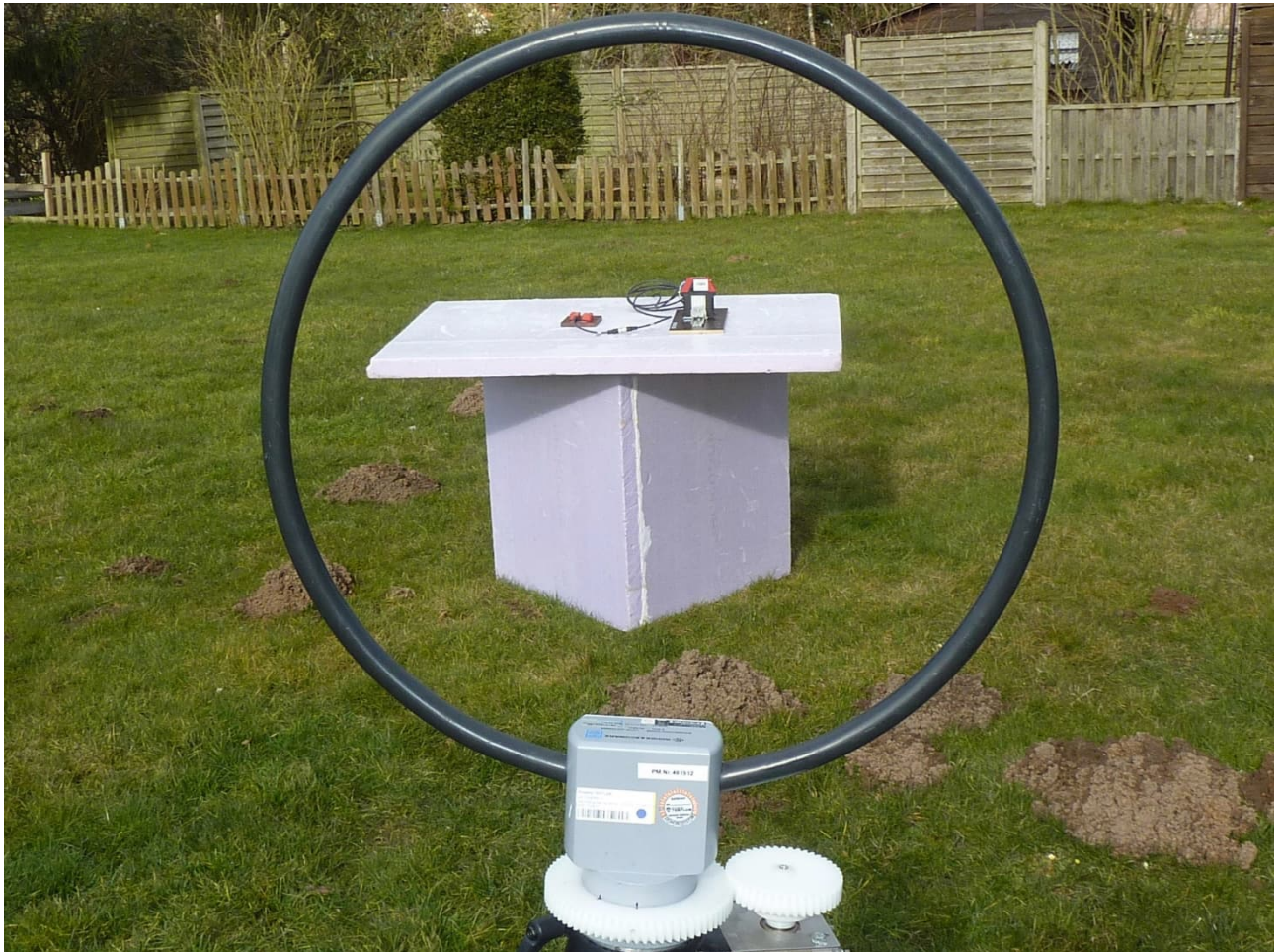
Test setup outdoor test side <30 MHz
