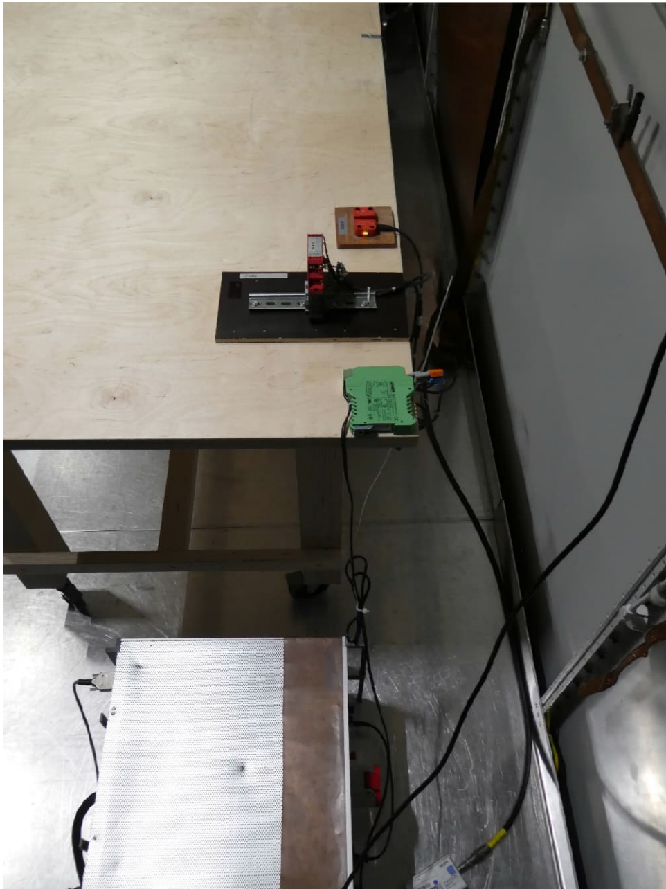
Test setup AC power line conducted emissions EUT 1
