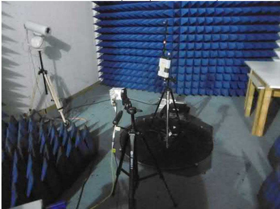
Anechoic chamber (Test setup for 18 GHz – 40 GHz)
