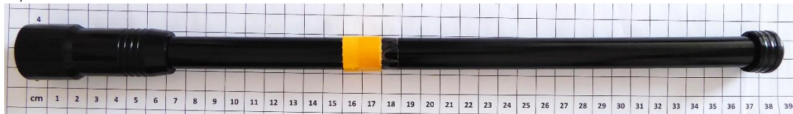
TX antenna, 9.0 dBi 5 GHz
