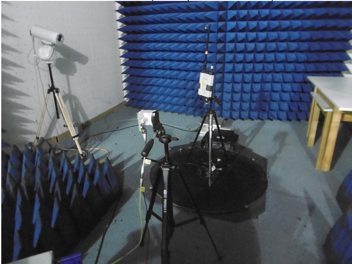
Anechoic chamber (Test setup for 18 GHz – 40 GHz)
