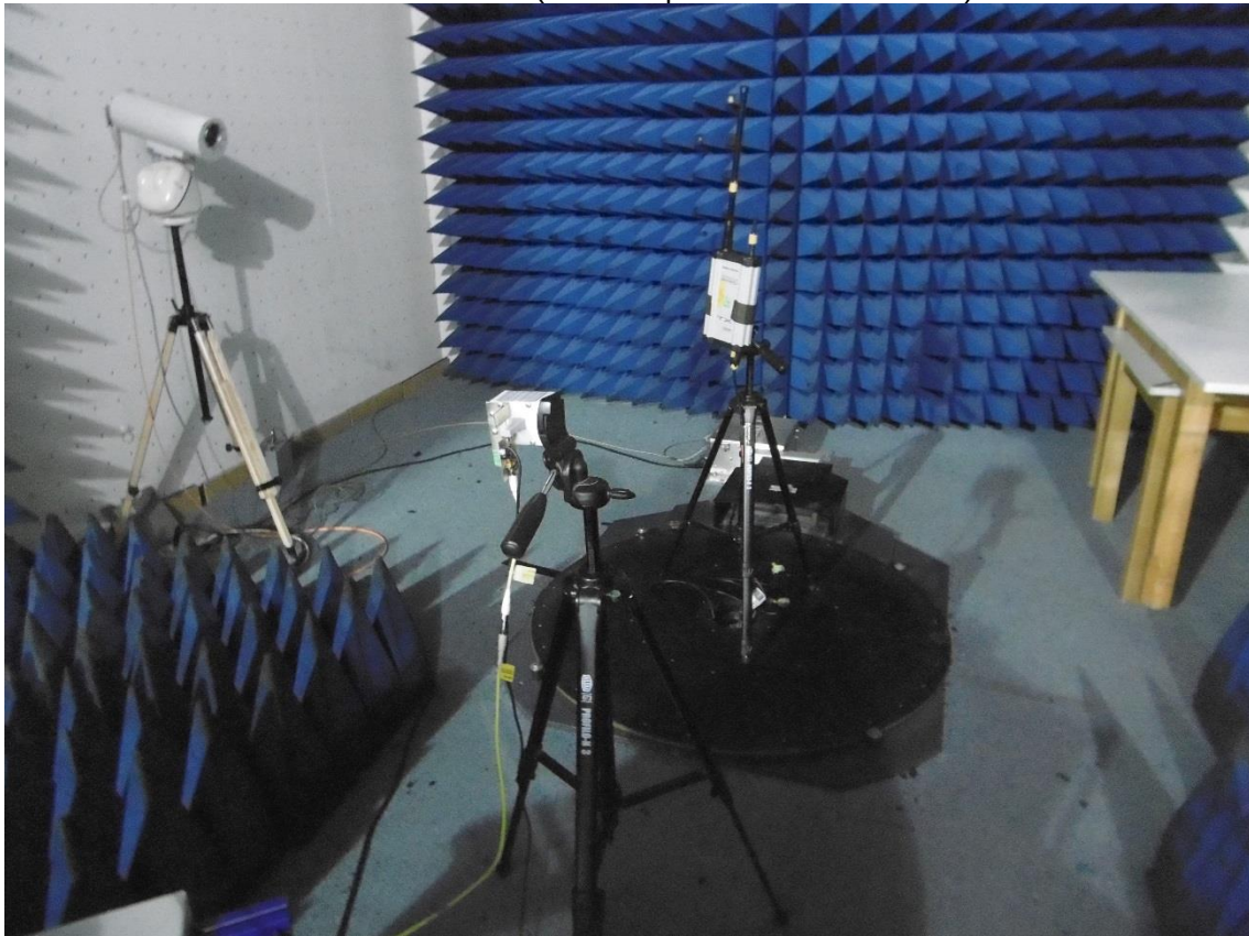
Anechoic chamber (Test setup for 18 GHz – 40 GHz)
