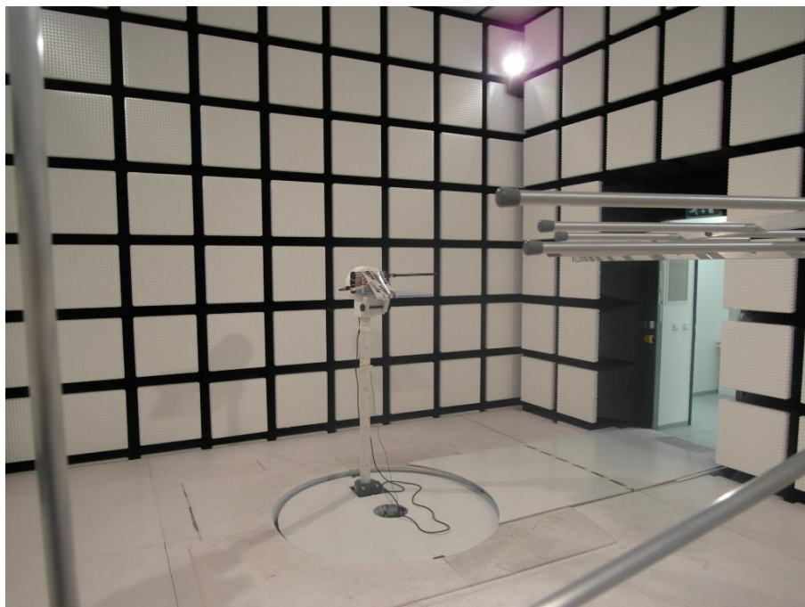
Photo 4 (RSE set-up / Fully-anechoic chamber):
