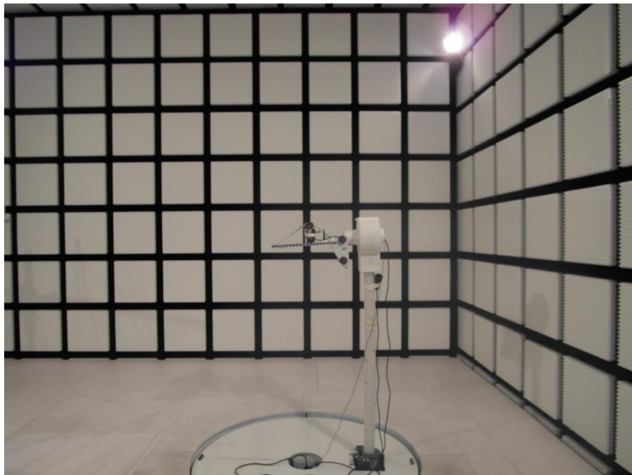
Photo 2 (RSE set-up / Fully-anechoic chamber):
