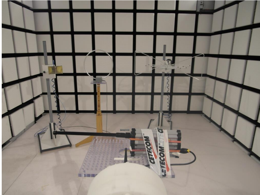
Photo 1 (RSE set-up / Fully-anechoic chamber):
