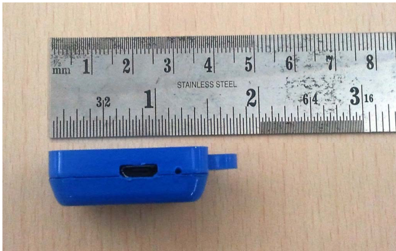
Figure 3: Photograph of EUT – Side View showing the USB connector
