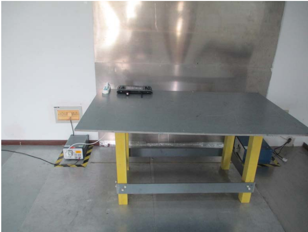
Conducted Emissions Test Setup – Front View
