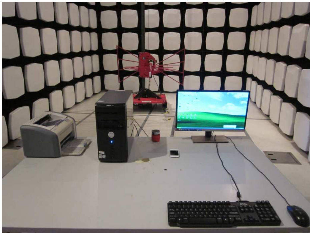
Measurement of Radiated Emission Test Set Up
