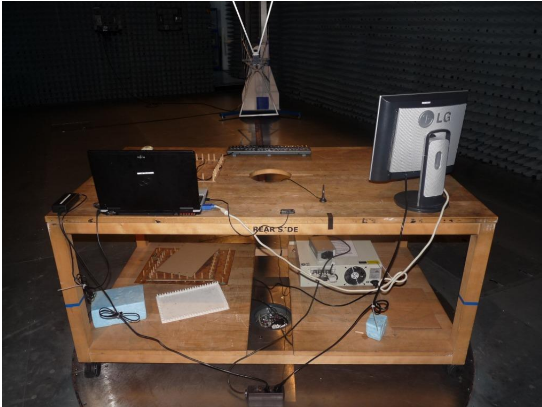
Photo 4: Test setup for radiated measurements (AC Port (power line), unintentional radiator §15) computer peripheral Setup.
