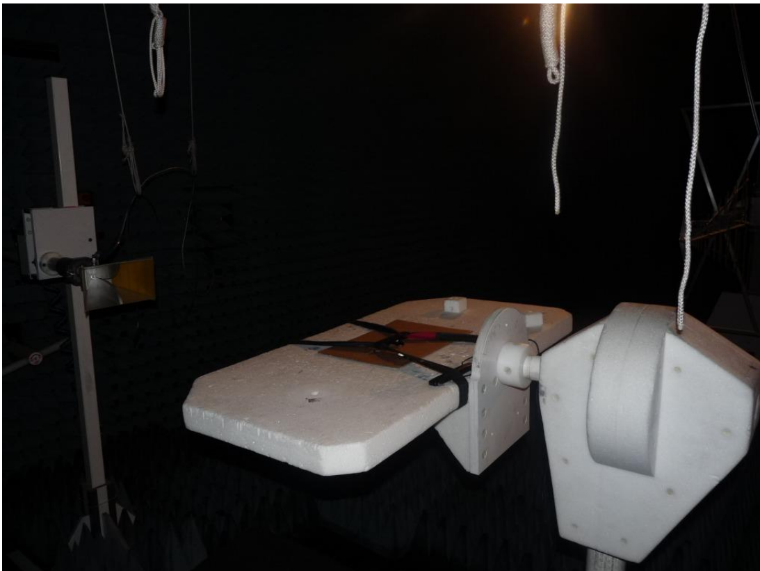
Photo 4: Radiated test setup used for FCC15.247 1GHz-25GHz.
