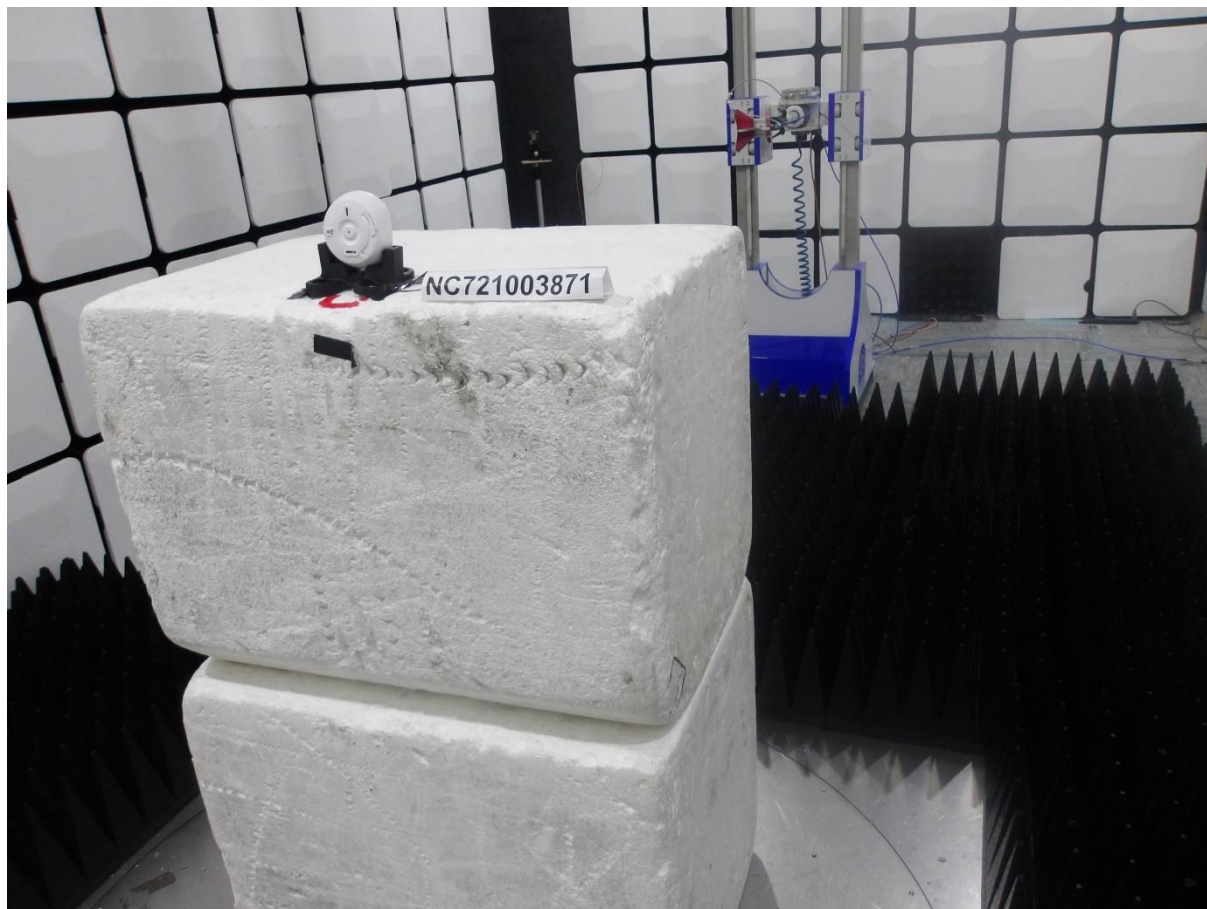
Photo 1.2-18 – Radiated Emissions Test Setup Photos – above 1 GHz – Rear View
