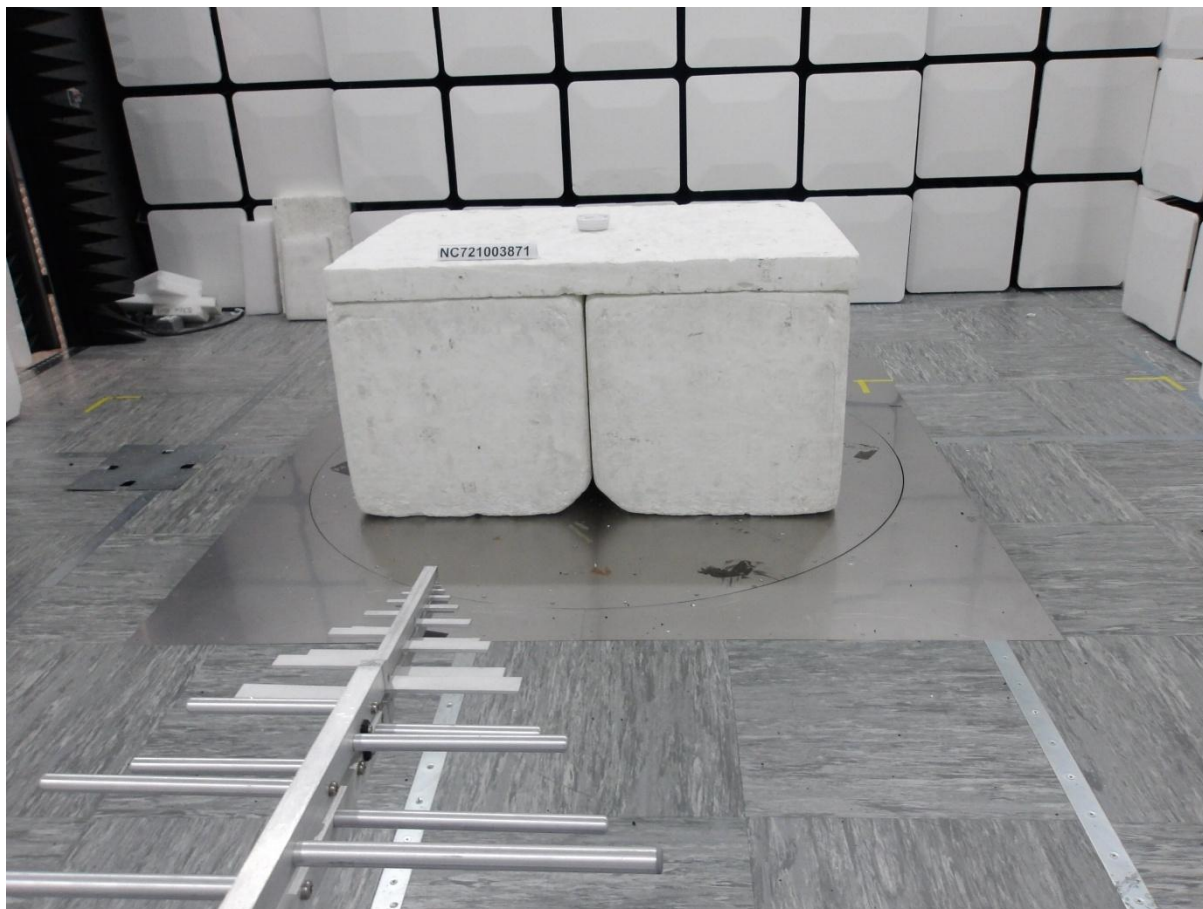
Photo 1.2-3 – Radiated Emissions Test Setup Photos – 30 MHz-1 GHz – Front View
