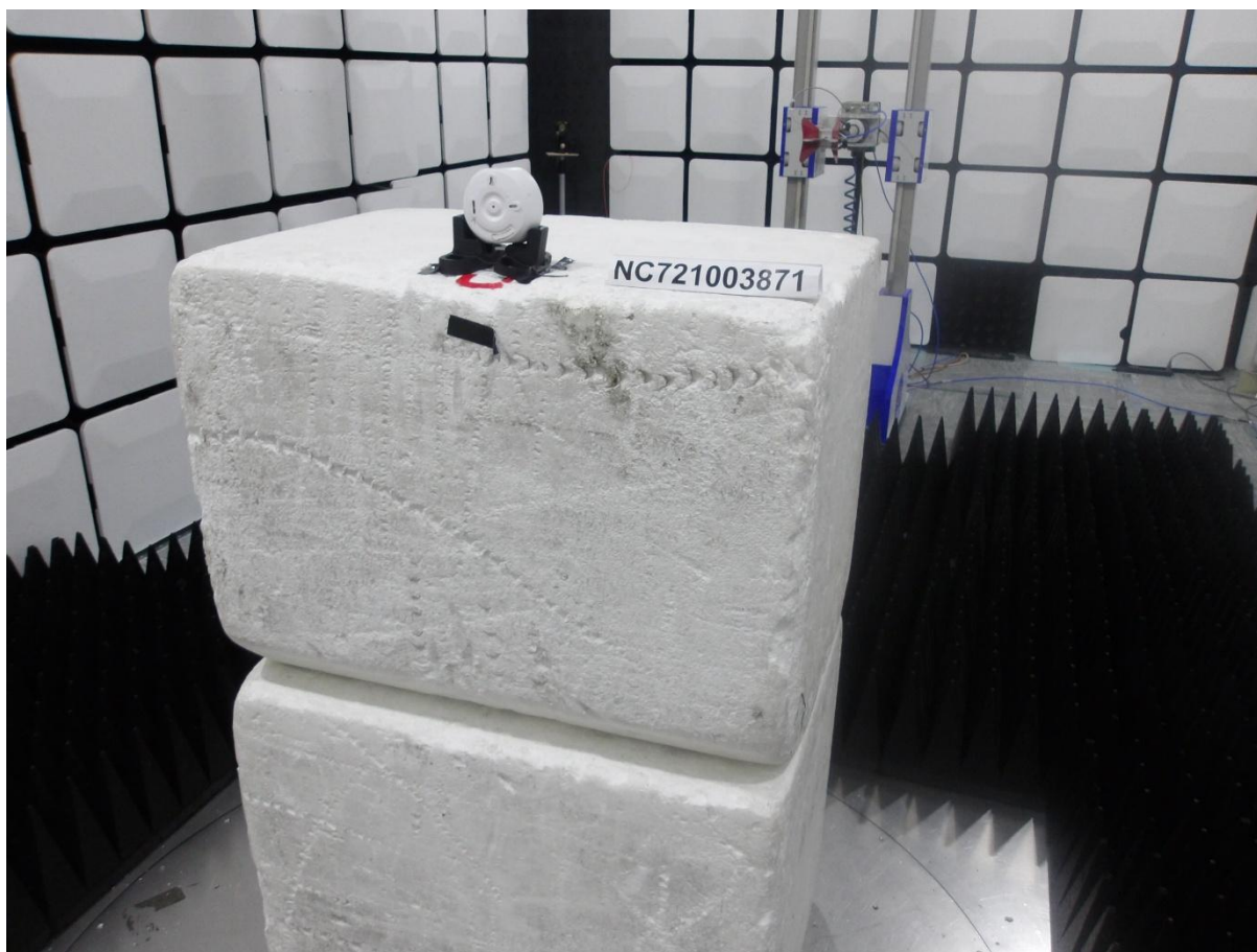
Photo 1.2-12 – Radiated Emissions Test Setup Photos – above 1 GHz – Rear View
