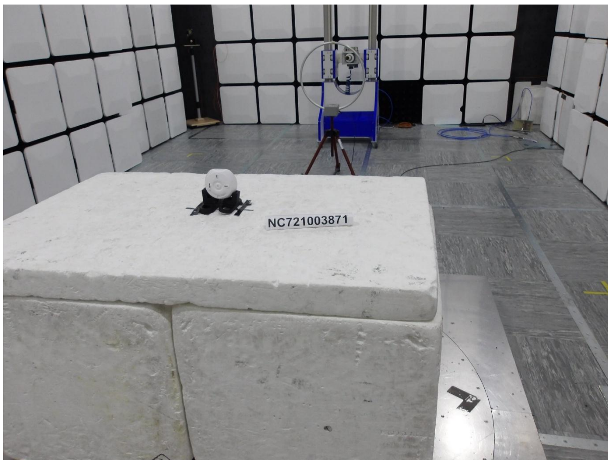
Photo 1.2-8 – Radiated Emissions Test Setup Photos – below 30 MHz – Rear View
