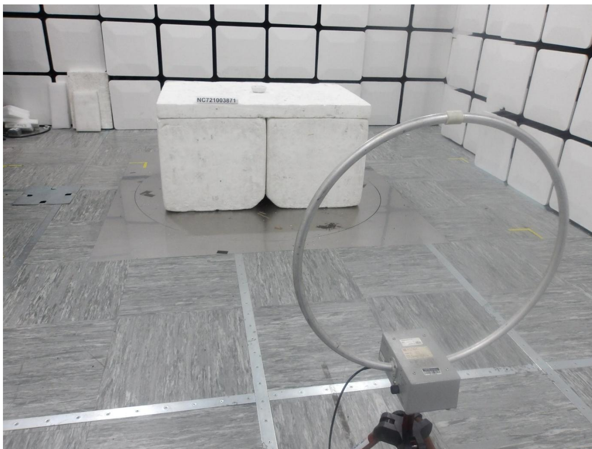
Photo 1.2-1 – Radiated Emissions Test Setup Photos – below 30 MHz – Front View
