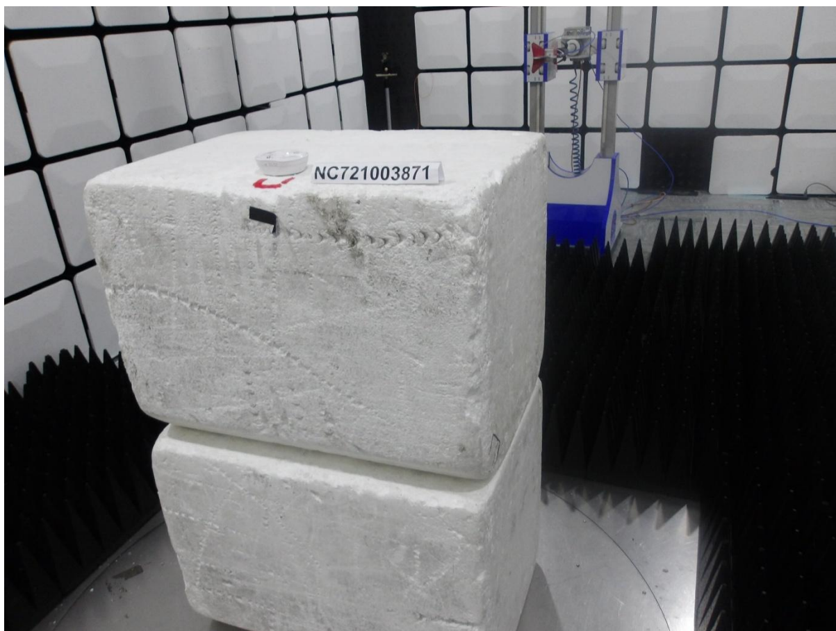
Photo 1.2-6 – Radiated Emissions Test Setup Photos – above 1 GHz – Rear View
