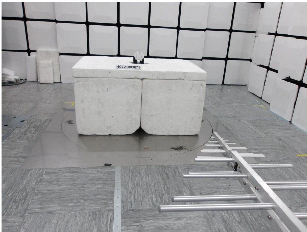
Photo 1.2-9 – Radiated Emissions Test Setup Photos – 30 MHz-1 GHz – Front View
