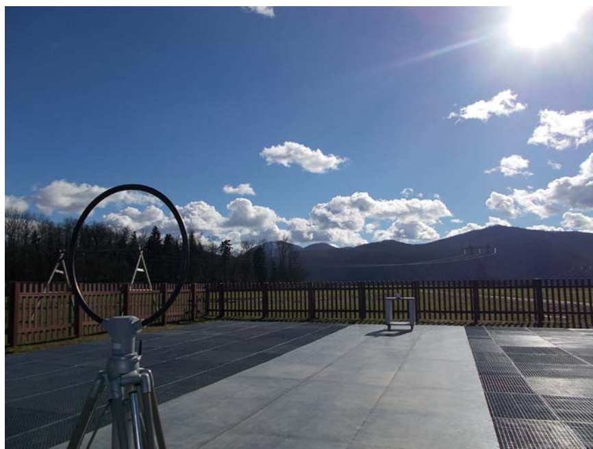
Figure 2: Radiated emission test – OATS measurements
