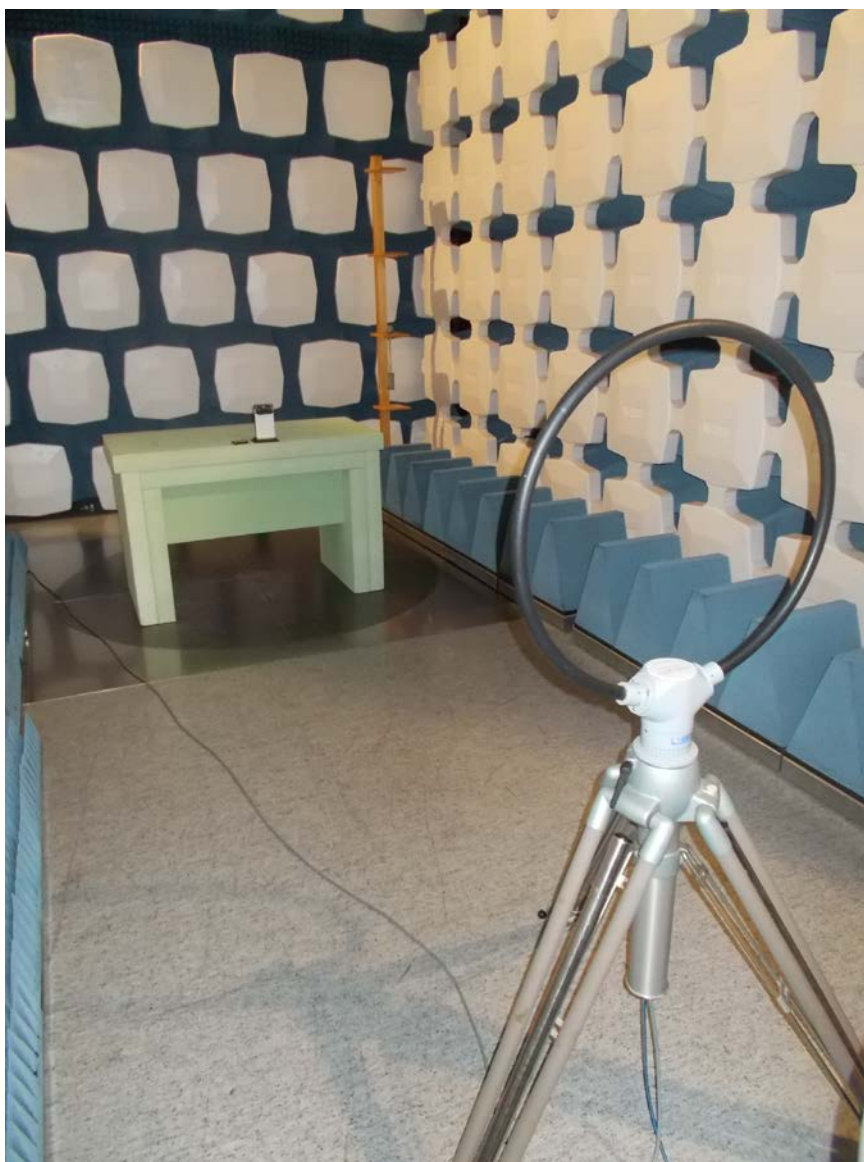
Figure 3: Radiated emission test – below 30 MHz
