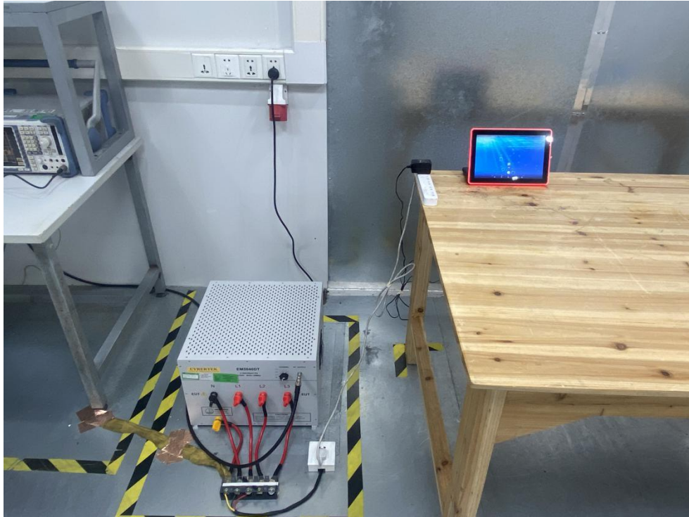
Photo of Conducted Emission Test
