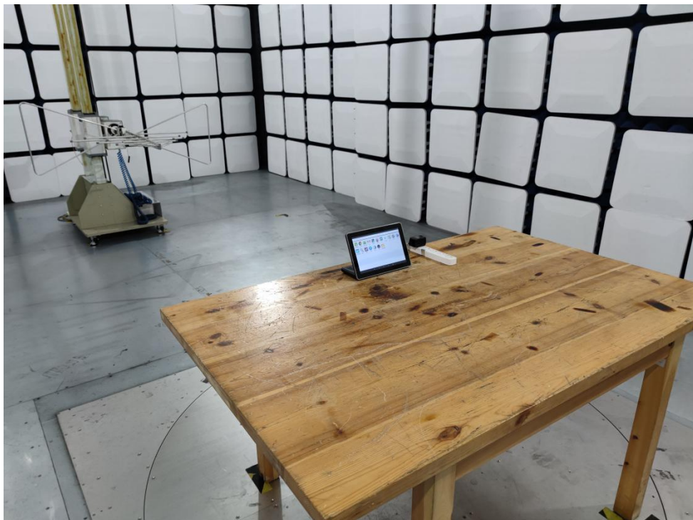
Photo of Radiation Emission Test
