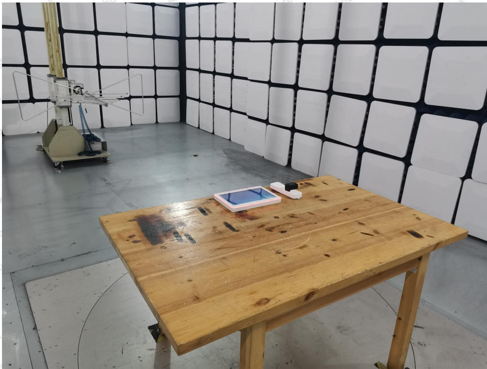
Photo of Radiation Emission Test
