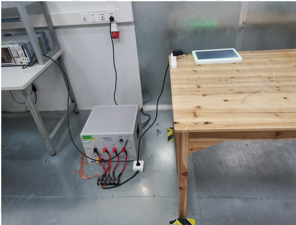
Photo of Power Line Conducted Emission Test
